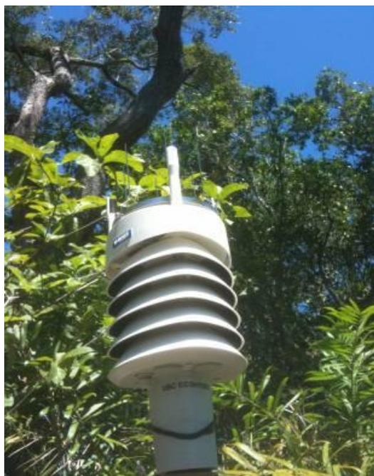
**Figura 8** – Transmissor meteorológico (modelo WXT520, Vaisala Inc., Helsinki, Finland).
