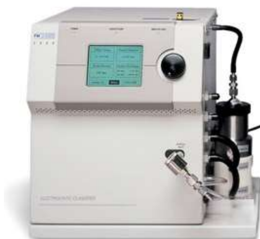
Figure 4. Electrostatic aerosol particles are charge-neutralized, size-classified by electrical mobility in a DMA, and counted by a Condensation Particle Counter (CPC), allowing the measurement of particle number size distributions (Inc., 2026)
