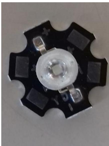
**Figura 22.** LED 850 nm, 3 Watts (Autor).
