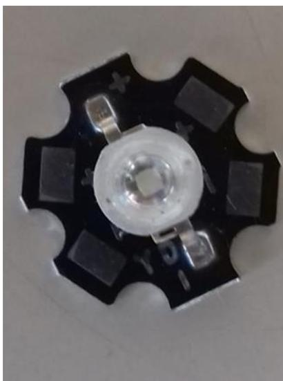
**Figura 20.** LED 660 nm, 3 Watts (Autor).
