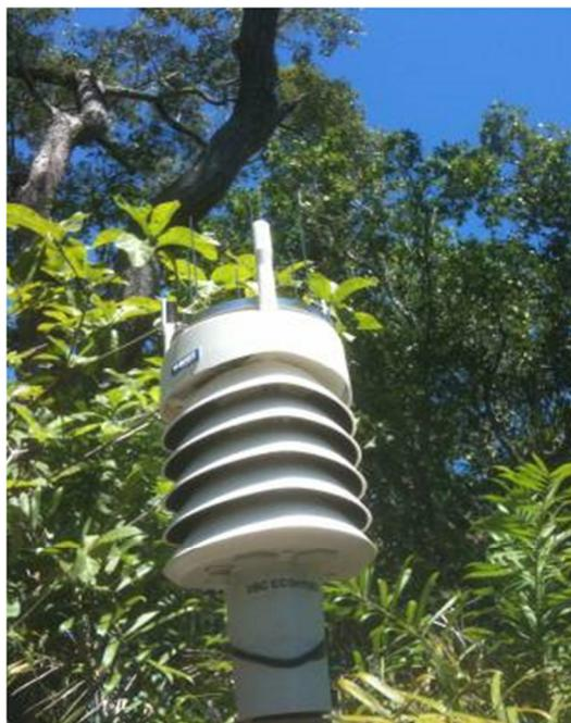
**Figura 3** - Sensor meteorológico (modelo WXT520, Vaisala Inc., Helsinki, Finland).
